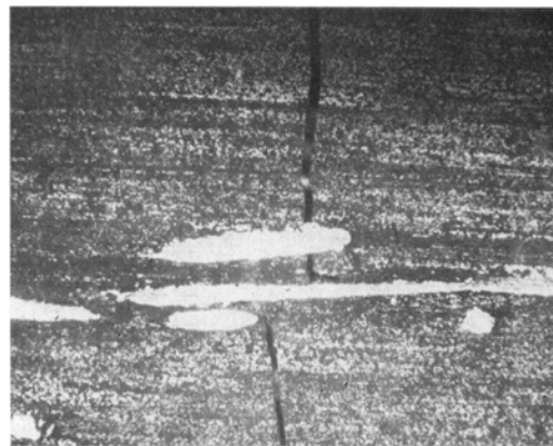
Figure 6 Crack branching and deflection at fibres.
